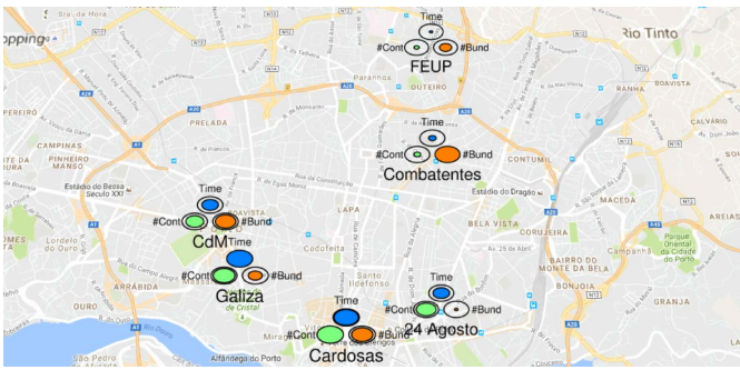
Fig. 11. Performance of I2V collection of UrbanSense DCUs data at locations served by BusNet nodes. Per location, the number of OBU-DCU contacts (left), total contact time (top), and number of exchanged bundles (right) are shown as a ratio to the network's maximum values (black circles).
